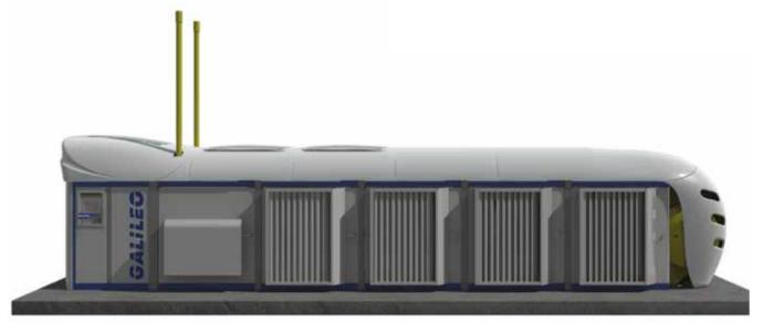
Cryobox® has an adjustable production capacity of up to 9 013 gpd (gallons per day). The high-pressure, thermodynamic cycle of the Cryobox converts natural gas to the liquid state as temperatures are reduced to less than -225 °F . This multi-stage compression process includes a "boil-off" recovery system which eliminates all gas-venting usually associated with LNG storage and loading facilities. This process avoids gas waste while complying with all safety and ecologic regulations.
